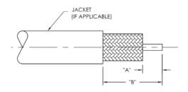
**1.** Trim cable to dimesions shown. Remove any burrs from outer and center conductor.
